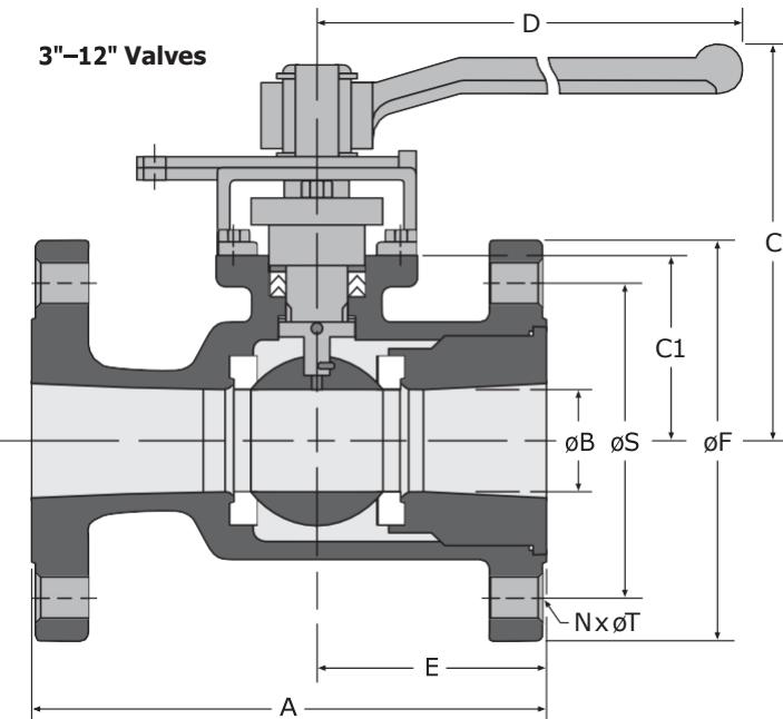
**NOTE:** Gear Operators are suggested on size 10" and 12" valves.
